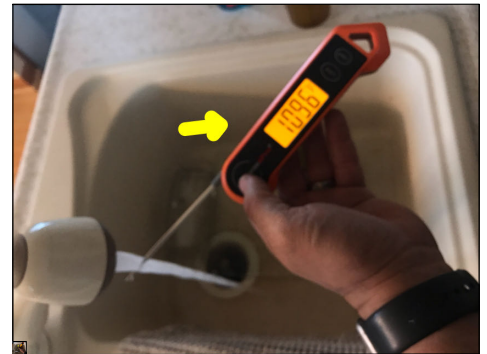
Temperature reading of the hot water during the time of the inspection. The approximate temperature of the hot water was 109 degrees Fahrenheit.
