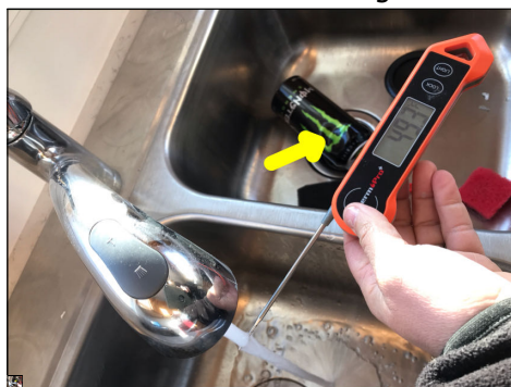
Temperature reading of the hot water during the time of the inspection. The approximate temperature of the hot water was 48 degrees Fahrenheit. There was no hot water through the house on the day of the home inspection.
