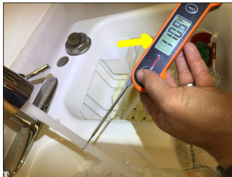
Temperature reading of the hot water during the time of the inspection. The approximate temperature of the hot water was 110 degrees Fahrenheit.
