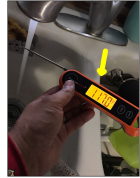
Temperature reading of the hot water during the time of the inspection. The approximate temperature of the hot water was 117 degrees Fahrenheit.
