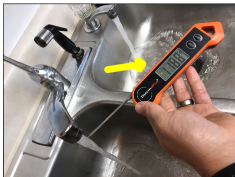
Temperature reading of the hot water during the time of the inspection. The approximate temperature of the hot water was 118 degrees Fahrenheit.
